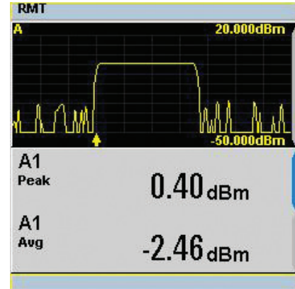
Figure 12. Effects of VBW on power meter measurements of a radar with fast-rising pulse edge.
